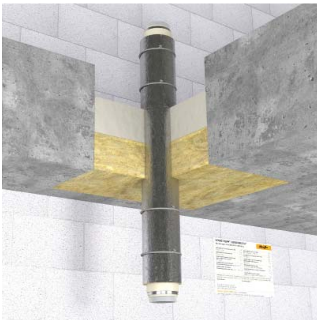
1 = Rigid floor, 2 = min. 50mm thick layer of HENSOTHERM® GM 2000, 3 = Mineral fibre board, 4 = Glass wool insulation, 5 = Aluminium-composite pipe
