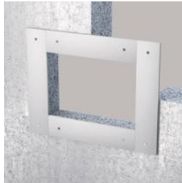
Fig. 2: Board frame for rigid floor and flexible wall (arranged either on one side or both sides, thickness of the board frame per side, max. 50 mm)
